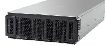
technologies developed based on a holistic view of devices, platform and their interactions. The first patented technology reduces vibration-induced performance degradation, while the second patented technology overcomes the cooling issues by introducing cool air into the middle of the platform. Both these technologies contribute to long-term reliability.
